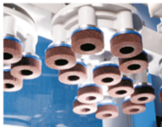
Deburring discs FAPI-TRIM used on a planetary head system
