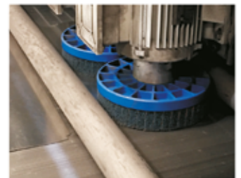
Deburring discs FAPI-250 used on a Loewer DiscMaster 4TD
