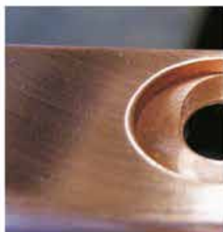
Workpiece before and after treatment with a deburring disc FAPI-M14 SAND on an angle grinder
