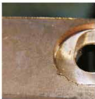
Workpiece before and after treatment with a deburring disc FAPI-M14 SAND on an angle grinder
