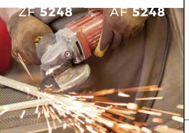
commonly used in the plastic industry as a mold release agent, **zinc stearate** is a powerful metal soap that repels water and acts as a lubricant. When applied on the abrasives, zinc stearate **creates free flow** between the grains.
