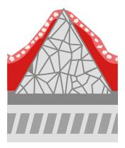
Crystal structure designed to reveal **sharp edges** while grinding down.
